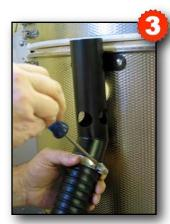
3) Secure one end of the black hose to the bottom of the exhaust stack using one of the 5cm clamps.
