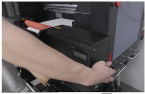
Install the back core and tighten the screws
