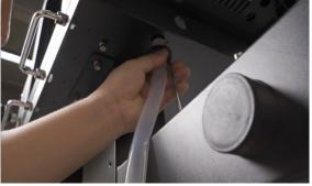
Trim the waste ink hose to match the height of the waste ink bottle. Turn on the waste ink level alarm.
