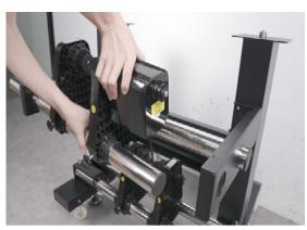
Tighten the screws to fix the take-up system on both sides
