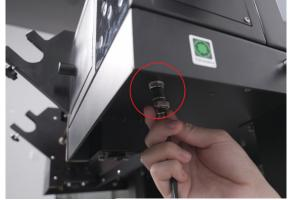
Install the waste ink bottle bracket Connect the waste ink tube
