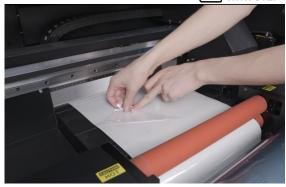
Use a tape to connect the film to the back
